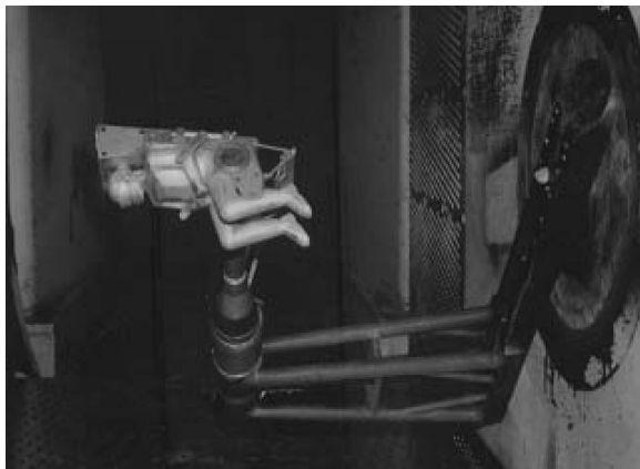
Fig. 2 Model installation and position in wind tunnel.
